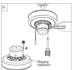
Remove shipping stabilizers from motor assembly.
