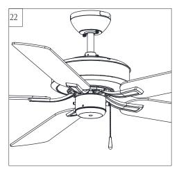
Install fan pull chains to preassembled pull chain on fan. Pull chain provided.
