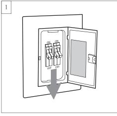
Before you begin installing the fan, Switch power off at Service panel and lock service disconnecting means to prevent power from being switched on accidentally. When the service disconnecting means cannot be locked, securely fasten a warning device, such as a tag, to the service panel. Use AC 120V/60HZ power supply only.
