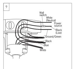
Make wiring connections using wire connectors provided as indicated above. White from fan to White (Neutral) from house. Black and Blue from fan to Black (Live) from house. Connect all green grounded wires to Grounded wire from House. Make sure that no filaments are outside of the wire connectors.
