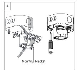
Install the mounting bracket onto the outlet box.
