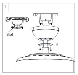
Lift Canopy allowing the 2 studs to protrude through the canopy. Next lift the cover ring and install knurled nuts as shown. Tighten the knurled nuts securely. The canopy should adjust for any irregularity in the ceiling or Outlet box.
