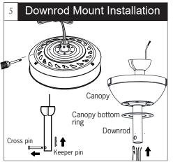
Partially loosen downrod set screws from voke at top of motor assembly. Remove preassembled cross pin and keeper pin from downrod. Place downrod over canopy and canopy bottom ring. Thread lead wires and safety cable from motor assembly through downrod.
