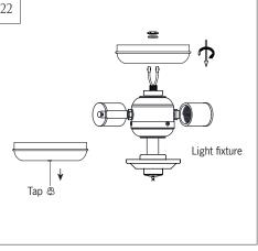
Remove the tap from bottom of the switch housing cap.
