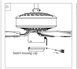
Remove switch housing cap by removing the set screws. Keep screws.
