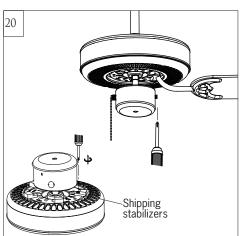
Remove shipping stabilizers from motor assembly.
