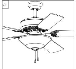
Install fan and light kit pull chains to preassembled pull chains on fan. Pull chains provided.
