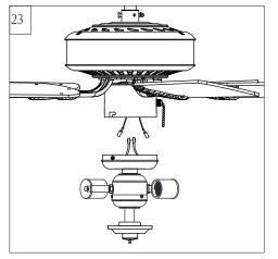
Connect light lead wires. White to white, blue (or black) to black (or blue). Make sure the quick connectors are clasped firmly.
