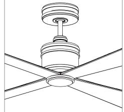
Lift canopy up, aligning its keyhole slot with the preassembled screw on mounting bracket and twist counterclockwise to lock in place. Reinstall the screw removed in step 16 and tighten all screws securely. Attach canopy bottom cap onto canopy by aligning its notch with the screws on mounting bracket and twist clockwise till tight.
