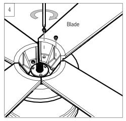
Place motor assembly on a suitable area of Styrofoam and install blades onto motor with set screws provided. Tighten all screws securely.
