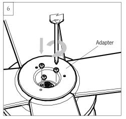
Install an adapter onto the plate on the motor using the set screws removed on last installation step.
