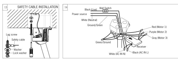
Safety cable must be installed into the house structure using 3" lag screws, washers, and lock washers provided, required for outdoor applications and in Canada (All fans installed in Canada), and for USA fan and light kit combinations over 35lbs.
