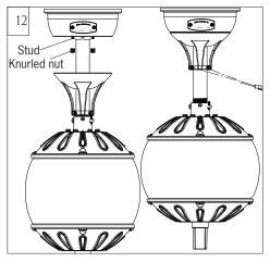
Lift Canopy allowing the 2 studs to protrude through the canopy, and then install knurled nuts as shown. Knurled nuts provided. Tighten the knurled nuts securely. The canopy should adjust for any irregularity in the ceiling or Outlet box.
