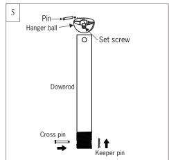
Remove hanger ball from downrod by loosing the set screw and removing the pin as shown in illustration. Keep parts. Remove preassembled keeper pin and cross pin from downrod.
