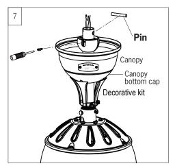
Place decorative kit canopy bottom cap and canopy over lead wires, safety cable and downrod, and then replace the hanger ball.
