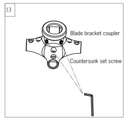
Partially loosen the countersunk set screws on the coupler of blade bracket. Use the Allen wrench provided.
