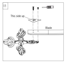
Install blade onto blade bracket with a top plate by 3 blade screws provided. Tighten screws securely. Repeat this process for remaining blades.
