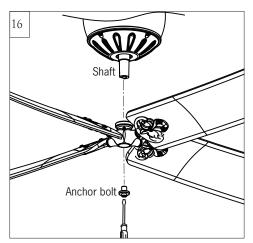
Slip the blade assembly on the shaft. Install an anchor bolt **counterclockwise** to fix the blade assembly in position. Tighten the bolt securely.
