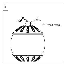
Partially loosen downrod set screw from yoke at top of the motor assembly.
