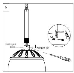
Thread lead wires and safety cable from motor assembly through downrod. Install downrod. Thread downrod into the yoke on top of fan until the holes on downrod are aligned with the holes on the yoke, and then install cross and keeper pins. Tighten the downrod set screw. **Caution**: To avoid damaging of lead wires from downrod installation, make sure the lead wires and safety cable are not twisted when install the downrod.
