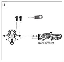
Insert a blade bracket into the coupler. Align the holes on the coupler with the screw holes on the blade bracket, and then fix the blade bracket with set screws provided. Tighten screws securely. Repeat this process for remaining blade brackets.
