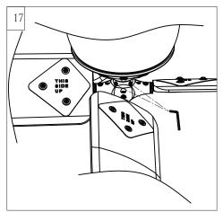
Fix the blade assembly with the countersunk set screws using the Allen wrench. Allen wrench provided.
