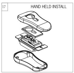
Place battery cover over battery compartment and buttons. Place remote over 2 pins on front cover. Attach cover of remote by placing over 4 pins and snapping into place.
