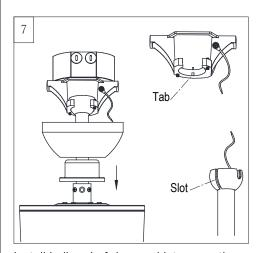
Install ball end of downrod into mounting bracket opening. Align (engage) slot on ball with tab on mounting bracket. **Warning:** Failure to align slot on ball with tab may result in serious injury.
