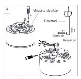
Remove shipping stabilizers from motor. Partially loosen downrod set screws from yoke at top of motor assembly. Remove preassembled cross pin and keeper pin from downrod.
