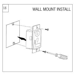
Install wall control unit to outlet box using machine screws provided.
