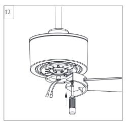
Install blade with screws provided, aligning each of the holes as shown and tighten all screws securely. Repeat this process for remaining blades.
