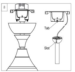
Install ball end of downrod into mounting bracket opening. Align (engage) slot on ball with tab on mounting bracket. **Warning:** Failure to align slot on ball with tab may result in serious injury. **Important:** If using the angle mount, make sure open end of mounting bracket is installed facing the higher point of the ceiling and make sure the ceiling angle is not steeper than 20°. Longer downrod may be necessary allowing the fan blades to rotate without obstructions.
