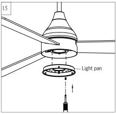
Attach the light pan onto the plate on motor, Place light pan over the lead wires from fan, aligning the keyhole slots on the light plate with the preassembled screws on the plate. Twist clockwise till lock. Reinstall the removed screw. Tighten all screws securely.
