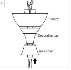
Place downrod over canopy, decorative cap and voke cover. Thread lead wires and safety cable from motor assembly through downrod.
