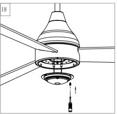
Attach the LED light fixture onto the light pan, aligning the keyhole slots on the LED light fixture with the preassembled screws on the light pan. Twist clockwise till lock. Reinstall the screw removed on the installation step 16. Tighten all screws securely.
