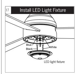
Connect the light lead wires from fan to LED light fixture with a quick connector as shown in the illustration. **Note**: Be sure quick connector clasped together completely.
