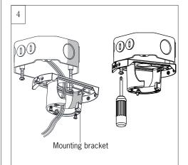
Install the mounting bracket onto the outlet box.
