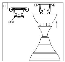
Lift Canopy, allowing the 2 studs to protrude through the canopy. Make sure the studs protruding from the bottom of the Mounting bracket are installed with threads all the way through the bracket.
