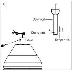
Partially loosen downrod set screws from voke at top of motor assembly. Remove preassembled keeper pin and cross pin from downrod. Keep parts
