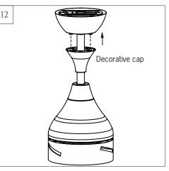
Install the decorative cap by locating its groove with the knurled nuts on canopy and turn clockwise till tight.
