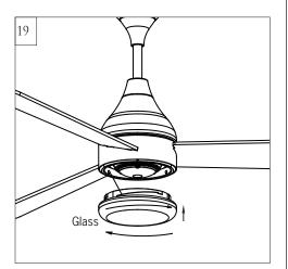
Attach the glass by locating dimples in light pan with grooves on the glass and twist clockwise until tight.
