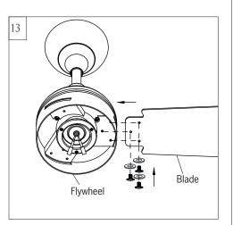
Insert blade into the slot on the flywheel. Install blade by the screws and rubber washers provided, aligning each of the holes as shown and tighten all screws securely. Repeat this process for remaining blades.
