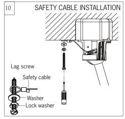
Safety cable must be installed into the house structure using 3" lag screws, washers, and lock washers provided, required for outdoor applications and in Canada (All fans installed in Canada), and for USA fan and light kit combinations over 35lbs.
