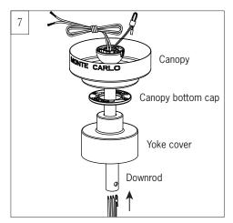
Place downrod over canopy, canopy bottom cap and yoke cover. Thread lead wires and safety cable from motor assembly through downrod.
