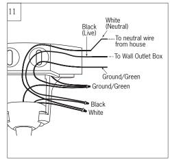
Refer to page 6 for wiring, installation and operation of Wall controller. Do not operate the fan or light until it is installed completely
