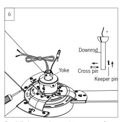
Partially loosen downrod set screws from yoke at top of motor assembly. Remove preassembled cross pin and keeper pin from downrod. Keep parts.
