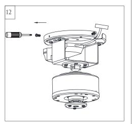
Loosen 2 screws across from each other and remove the other 2 preassembled screws from side of mounting plate (corresponding to installation step 13). Save screws for later use.
