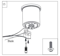
Align the 2 side holes on the blade with the screw holes on the motor. Install the blade by setting screws with washer provided. Repeat this process for other blades. Tighten all screws securely. The middle hole is for blade supporting plate installation on next step.
