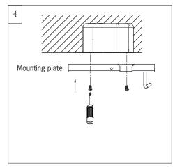
Remove the two set screws provided with the outletbox, aligning the holes of the mounting plate with the screw holes in the outlet box. Reinstall the 2 outlet box screws securely.
