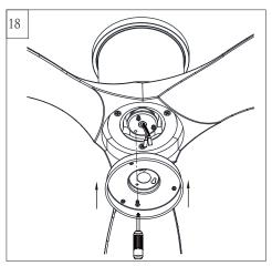
Place the lead wires from fan over the central hole of light pan Aligning the keyhole slots on the light pan with the preassembled screws on the plate. Twist clockwise till lock. Reinstall the screw removed in installation step 17. Tighten all screws securely.
