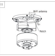
Pass the wifi antenna through the notch on the mounting plate and reach outside of the fan housing corresponding to the installation steps 13 and 14, then stick/fix it onto ceiling as shown in illustration on the installation step 14.
