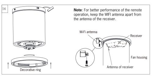
Attach decorative ring by locating the head of set screws on housing with grooves in the decorative ring and twist clockwise till tight.
