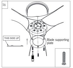
Align the holes on the blade supporting plate with the middle hole of the blades and install set screws provided. Tighten set screws securely.
