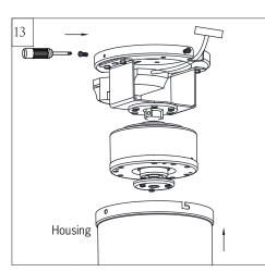
Attach housing onto mounting plate, aligning the keyhole slots on the housing with the screws on mounting plate and twist clockwise till tight. Reinstall the screw removed in step 12. Tighten all screws securely.
