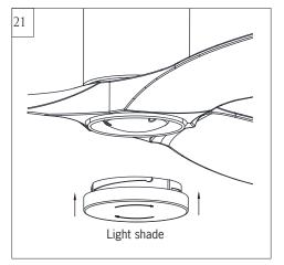
Attach light shade by locating dimples in light pan with grooves on the light shade and twist clockwise until tight.
