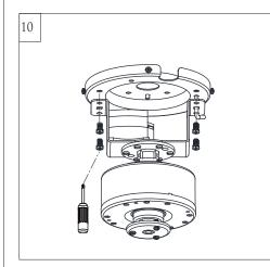
Lift motor assembly, aligning the holes on the plate on top of motor with the screw holes on mounting plate. Install set screws to fix them. Screws provided. Tighten all screws securely.
