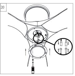
Connect white wire from fan to white wire from LED light fixture and then connect blue (or black) wire from fan to black (or blue) wire from LED light fixture. Be sure plugs connection clasped together completely. Attach LED light fixture onto the light pan, aligning the keyhole slots on the LED light fixture with the preassembled screws on the light pan. Twist clockwise till lock. Reinstall the screw removed in installation step 19. Tighten all screws securely.
