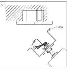
Hang motor assembly onto the hook on mounting plate for hands-free wiring and safety cable installation.
