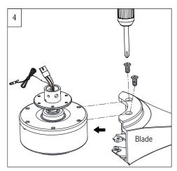
Place motor assembly on a suitable area of paper pulp for blades installation.
