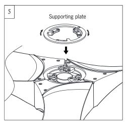
Flip the fan body with blades over and install the supporting plate.
