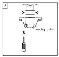
Use metal outlet box suitable for fan support and use only the screws provided with the outlet box (must support 35 lbs).
