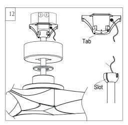
Install ball end of downrod into mounting bracket opening.
