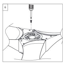
Install set screws onto blades with the supporting plate using screws provided.
