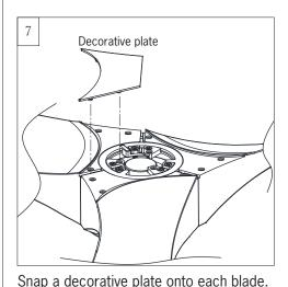
**Note**: Make sure they are engaged with the blades firmly to make the blades
