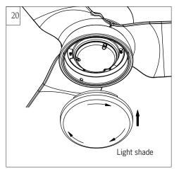
Attach the light shade by locating dimples in light pan with grooves on the light shade and twist clockwise until tight.
