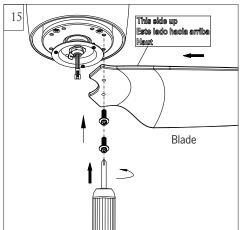
Install a blade to motor using the screws provided. Tighten screws securely. Repeat this process for remaining blade assemblies.
