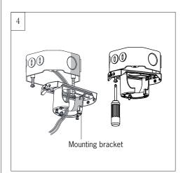
Install the mounting bracket onto the outlet box.
