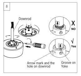
Spin the downrod into the yoke on top of fan until the hole with the arrow mark on downrod is close and aligned with the groove on top edge of the yoke, and then reinstall the screws securely.
