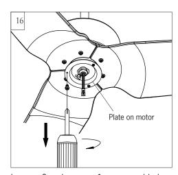
Loosen 2 and remove 1 preassembled screw from the plate on motor. Save screw for later use.
