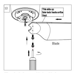
Align the holes on a blade with the screw holes on the motor, Install the blade using set screws provided. Repeat this process for other blades. Tighten all screws securely.
