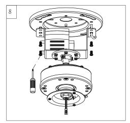
Attach motor assembly onto mounting plate.
